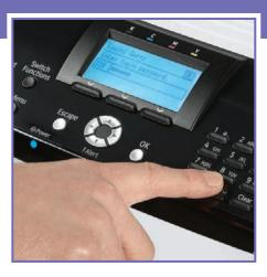
Locked Print\* enables secure, password-protected printing. The SP C430DN/SP C431DN Control Panel includes a 12-key alphanumeric keypad to make entering passwords easier.
